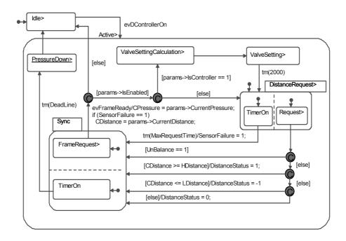
Figure 3 State chart of PI closed loop controller
