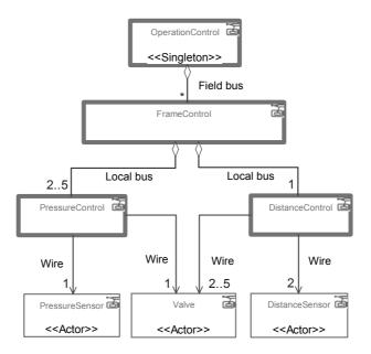
Figure 2 Class diagram of hydraulic press control
