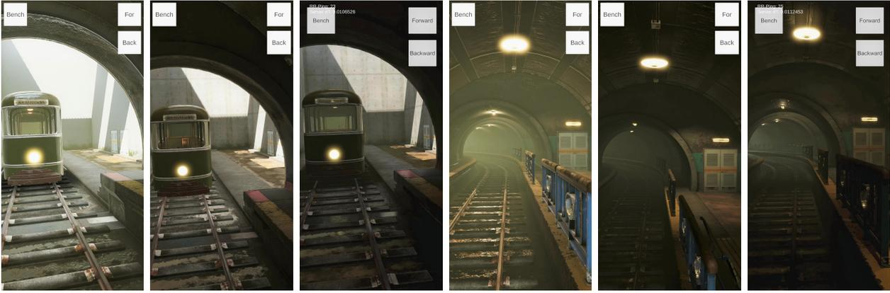
Figure 3: Comparison of two views of the full screen test with different rendering pipelines (twice from left to right: LWRP, LRP, RRP). The LWRP shows less details and uses only a simply lighting model. The RRP shows more details than the native rendering pipelines.
