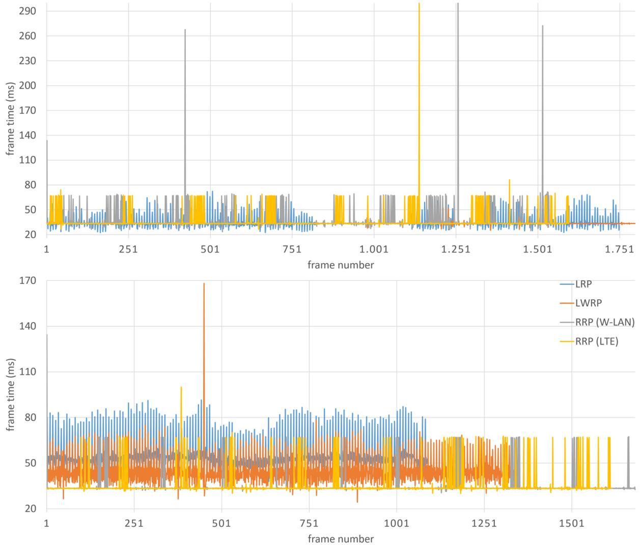
Figure 4: The frame times of the AR scene in HD1080 (top) and HD1440 (bottom). The RRP has several peaks compared to LRP and LWRP, which are related to transmission errors. Even with this peaks, the RRP shows a higher performance in HD1440.
