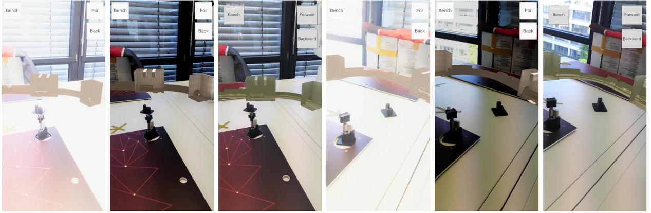
Figure 2: Comparison of two views of the AR object with different rendering pipelines (twice from left to right: LWRP, LRP, RRP). The real world view of the LWRP is overexposed due to the usage of linear color space for the Spotlight Tunnel and the used version of AR-Foundation, which can not handle a linear color space on the camera image.
