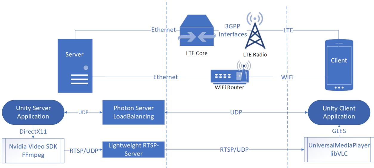
Figure 1: Overview of our remote rendering system. It uses either a W-LAN Router or a LTE Network with complete radio and core network.
