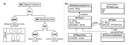
Figure 1: a) Example SFT. b) Meta model for SFTs.
