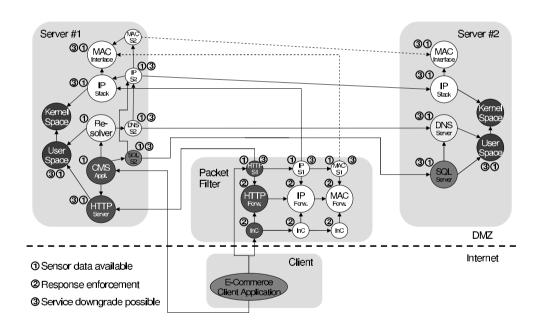
Figure 1: Example Dependency Graph of an e-commerce scenario with two DMZ hosts, different services and a packet filter for access control.
