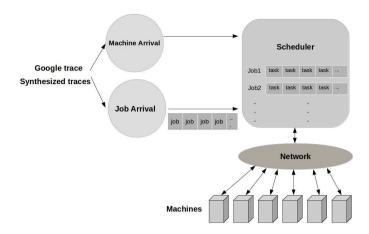
Figure 6: Architecture of simulation model.
