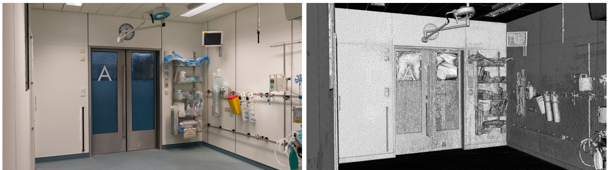
Figure 1: Textured mesh of an anaesthesia room that was generated by point cloud scans (left) and the visualization of the corresponding wireframe (right). The scene has to be segmented to develop interactive VR elements.
