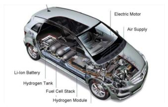
Figure 1: Vehicle with electric drive based on hydrogen fuel cell [CO12]
