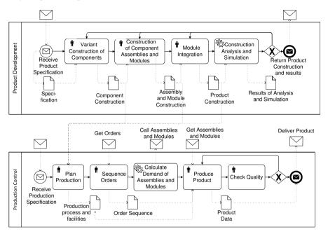
Figure 4: Process Modell of Product Development and Production Control
