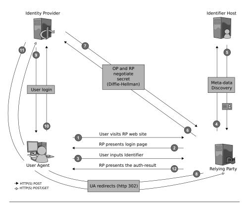
Figure 2: Typical OpenID Protocol Flow
