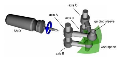
Concept of the smart mechatronic driver (SMD) adjusting the different axes of the mechanical positioning device to align the guiding sleeve with the planning data
