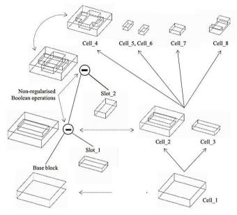
Figure 2: Feature model based on the cellular topology [MCG09]
