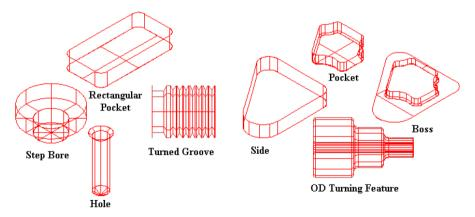
Figure 1: Common features of CAD/CAM applications [Image courtesy: FeatureCAM, 2008]
