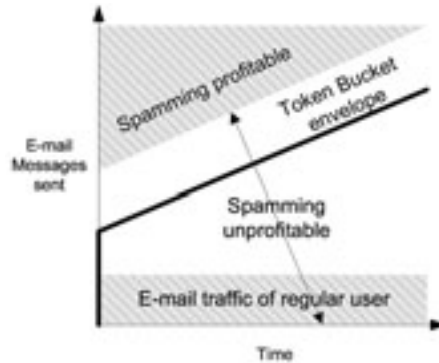
Figure 2: Token bucket envelope separating the region of regular e-mail traffic from the region of profitable spamming.
