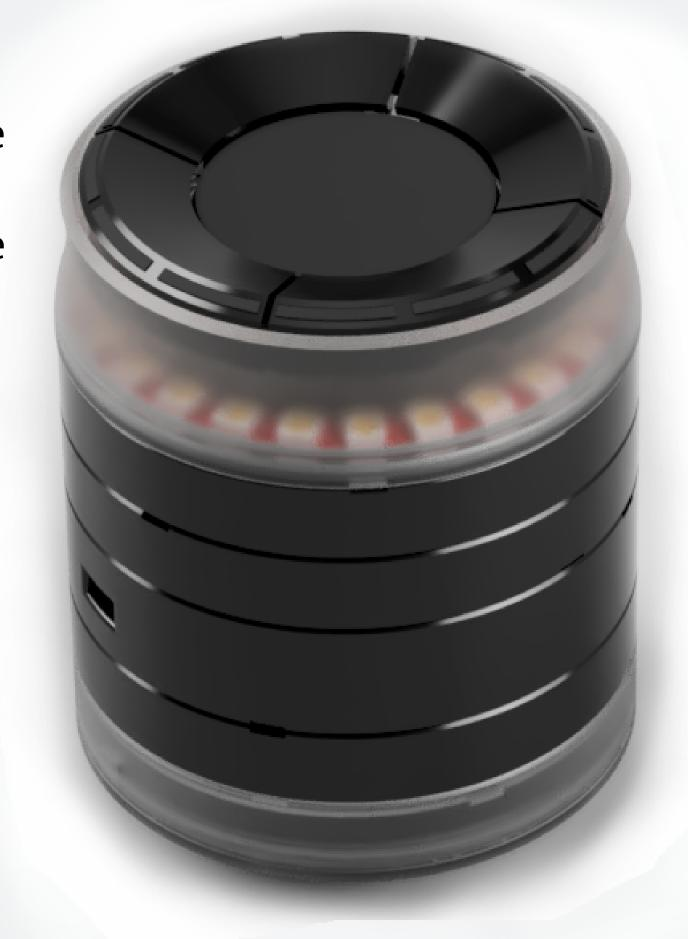
The circular top disc is a high resolution touchpad which acts both as a momentary click button and a fine grain touch input panel, the surrounding four circular button slices act as one capacitive touch and one click buttons each.. Relative position sensing is performed internally by two combined laser time-of-flight distance sensors and one 6-degrees-of-freedom inertia measurement unit.
