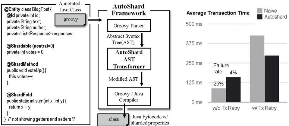
Figure 1: Compilation of an annotated Java class (left) with the AutoShard framework (middle). Evaluation of property sharding with 2,000 users incrementing 16 counters (right).
