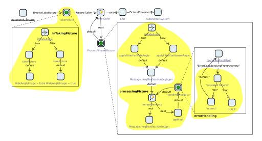
Figure 1: Behavioral model of the picture transmission process. Bottom right: a new error handling recovery mechanism.
