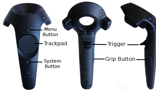
Fig. 1: The design of a controller of the HTC Vive with its buttons and their names.
