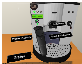
(b) The laser controller with the activated laser beam, a tooltip (pictogram of an empty cup) of a usable object (coffee machine button) is activated.
