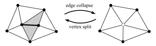
Figure 1: An edge collapse operation. The thick edge is collapsed to the unfilled vertex, the marked triangles are removed.
