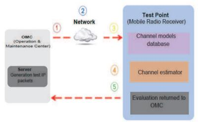
Figure 2: Functional model for channel classification in mobile networks
