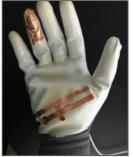
Glove with copper band to detect when the grasp is closed, and fingers touch the palm – electric circuit.
