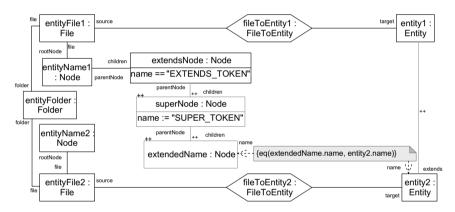
Figure 3: TGG rule creating an extends relationship and corresponding tree structure
