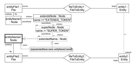
Figure 6: The new version of the TGG rule using binding expressions
