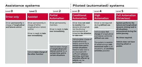
Figure 1: SAE levels for the automation of the driving task (Society of Automotive Engineers (SAE) International, 2014)
