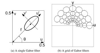
Figure 1: Representation of a single 2D Gabor filter (1a) and of a grid of Gabor filters (1b) in the frequency domain.
