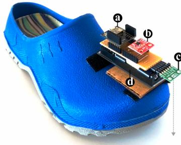
Figure 2: Hardware prototype mounted on an OR shoe with Velcro fastener consisting of a microcontroller with Bluetooth stack (a), gyroscope (b), distance sensor (c) and power supply (d).
