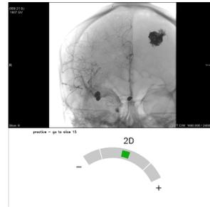
Figure 3: Graphical user interface showing medical image data on top and visual feedback for foot interaction at the bottom. A green cursor indicates the foot's position and shrinks to 60% of its size when lifting the foot.
