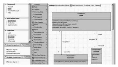
Figure 4: Structural view of a Component Specification
