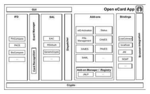
Figure 1: Extensible architecture of eID-client-platform
