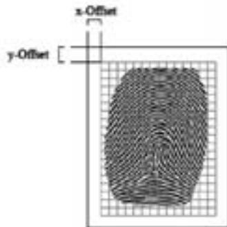
Figure 1: The tessellation of a fingerprint with an optional X- and Y-Offset.
