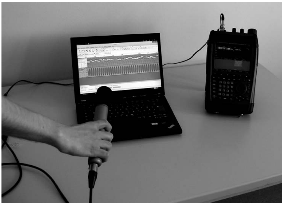
Figure 6: Locating the source of a covert audio signal with a mobile device (PR100)
