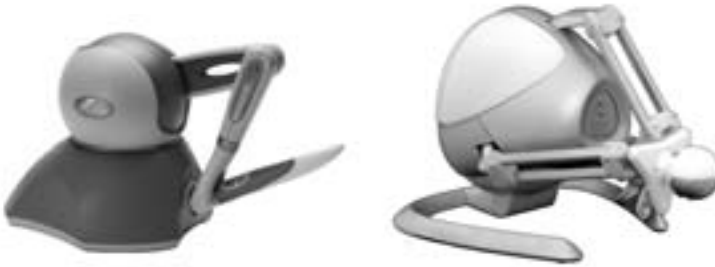
Figure 1: Haptic Devices: the SensAble PHANTOM Omni® is a serial 6DOF input, 3DOF output device ( http://www.sensable.com ), the NOVINT Falcon® is a parallel 3DOF input/output device ( http://home.novint.com/products/sdk.php ). Photos are courtesy of SensAble and NOVINT.
