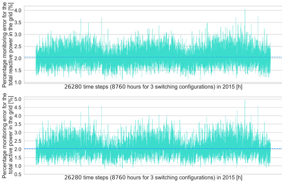
Fig. 8: Percentage error of the total estimated reactive and active power of the SimBench grid (2015)
