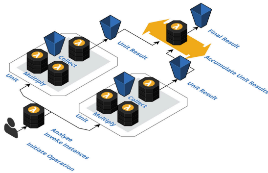
Fig. 1: Overview of our serverless processing architecture.
