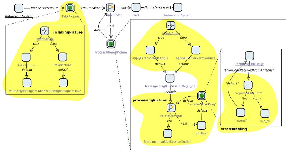
Figure 1: Behavioral model of the picture transmission process. Bottom right: a new error handling recovery mechanism.
