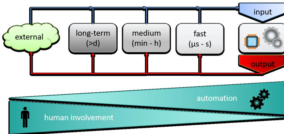
Figure 1: The input and output of a manufacturing step, sub-process, or process are controlled via feedback loops with various time horizons and a varying degree of automation.
