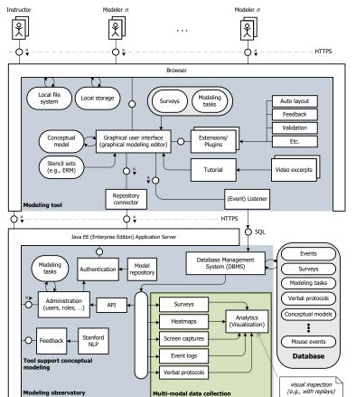
Fig. 1: Software architecture at the conceptual design level depicted using FMC (Fundamental Modeling Concepts [KGT06]). The green area represents the technical components of the multi-modal observation and data generation approach.
