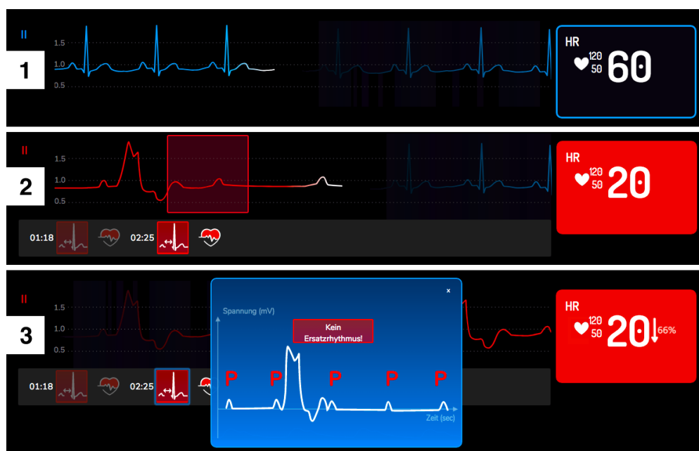
Figure 1: Different States of ECG Parameter of Prototype C during Scenario "Cardiac Arrhythmia (Phase 3)" 1: No Alarm, 2: Alarm State with Cue and Timeline, 3: Detailed View of an Event
