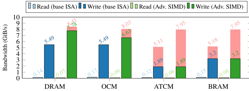
Fig. 1: Bandwidths of non-cacheable APU memory accesses (for the largest tested transfer size). ■ denotes unsustainable or short-term write bandwidth.
