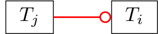
Fig. 1: Negator relationship between tasks T_j and T_i : If T_j is assigned, T_i must not be assigned
