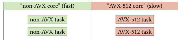
Figure 3: We employ core specialization to reduce remote AVX overhead [8]. If only some cores are allowed to execute AVX-512 instructions, tasks on the other cores will never execute at AVX-512 frequencies.
