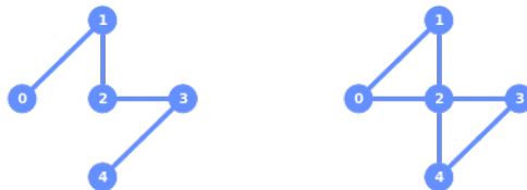
Fig. 2: Qubit coupling map of IBM Quantum Athens (left) and Yorktown (right) [IB20]
