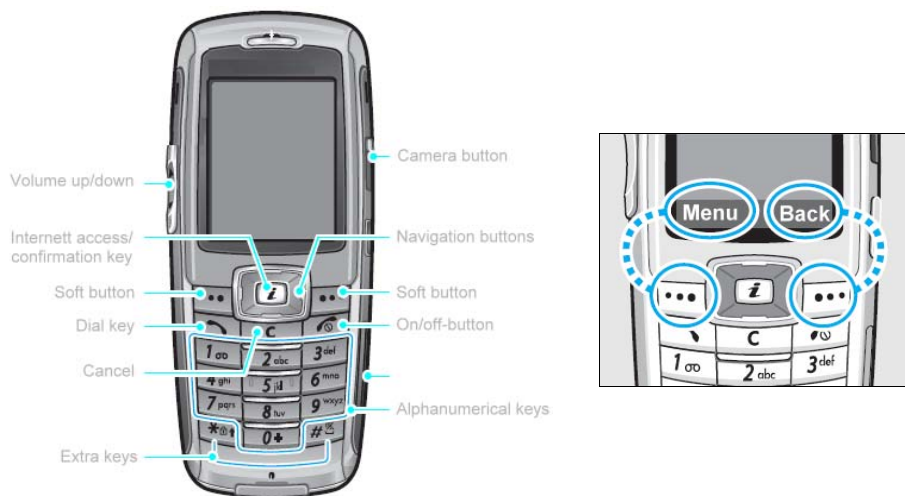
Fig. 2: Physical controls of a standard mobile phone (24 1-DOF controls) 2 ; mappings explained in the mobile phone manual (right)
