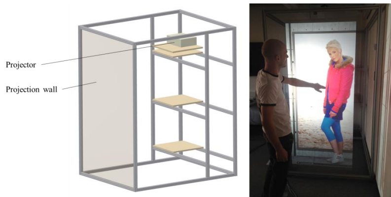
Figure 2: Prototypic Implementation (left: prototype construction, right: user interface with digital avatar)
