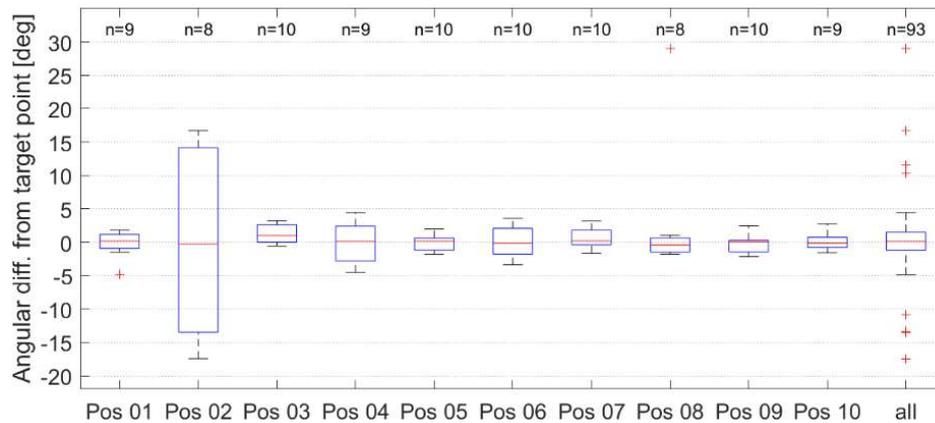
Fig. 4: Difference to the target orientation of the respective target point and all measurements.  $n < 10$  caused by triggering the safety module
