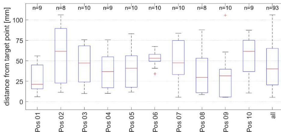
Fig. 3: Amount of the distance of the robot end position to the target points
