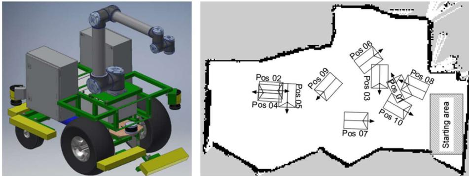
Fig. 1: 3D model of the mobile robot platform (left) and map of the test environment with start area, 10 target positions and orientations (right)
