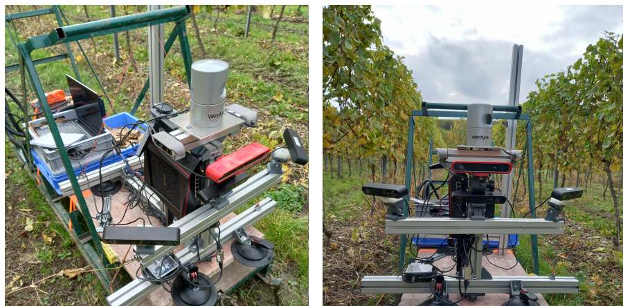
Fig. 5: Data recording for validation of the control and perception concepts. The sensor setup used on the robot is mounted to an experimental design to check the sensing quality. The Velodyne HDL32E laser serves as the ground truth for the stereo cameras.
