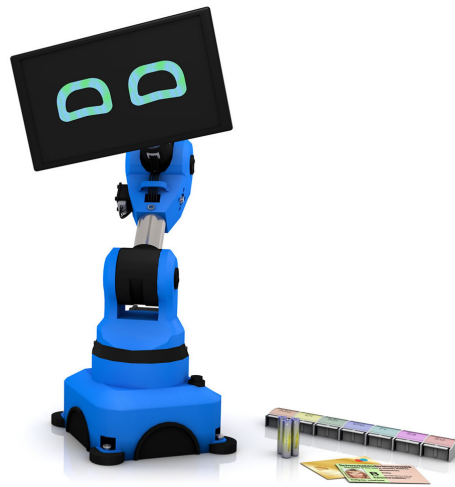
Fig. 1. Prototype 3D-Rendering of the envisioned interactive system: A very mechanical appearing social robot based on a robotic arm (compact 6-axis robotic arm) and a tablet computer. Depending on the desired mode, it can show two abstract stylized eyes (that can turn into different shapes and represent an abstraction of various facial expressions or emotions), as well as display video messages, live video streams or other relevant information.
