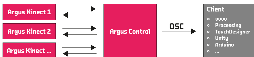
Figure 1: The architecture of Argus Vision.
