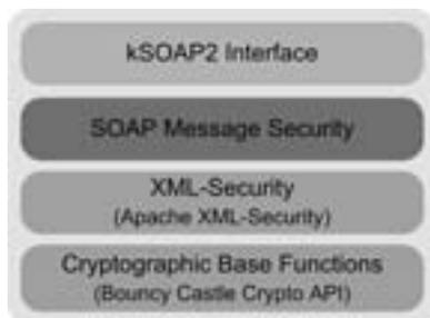
Figure 4: Extension of kSOAP2 for Security Features
