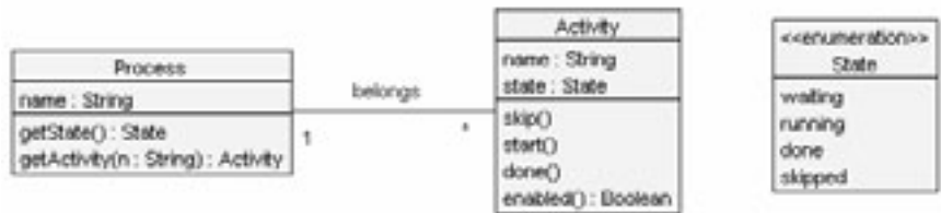
Figure 1: UML model for flat workflow specifications modeled in USE
