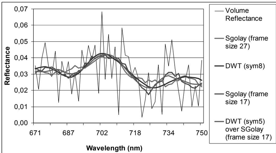
Figure 3. Comparison of noise removal filters for volumetric reflectance. The best performing filter is a combination of first Savitzky-Golay Filter with small frame size (e.g. 17) and then Discrete Wavelet Transformation with *Sym5* de-noising wavelet.
