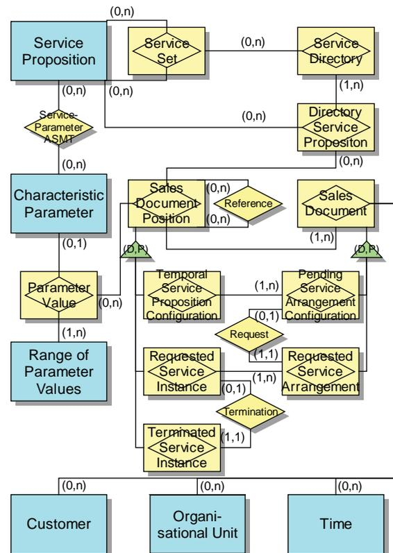
Figure 6: Data structure for service arrangement configuration [eERM]
