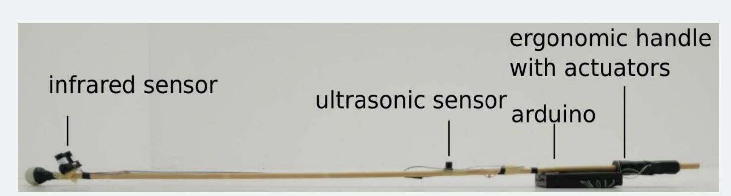
STIC mimics a typical white cane and is extended by an Arduino based system. It contains an infrared sensor to detect obstacles at ground-level and an ultrasonic sensor for head-level obstacles.
