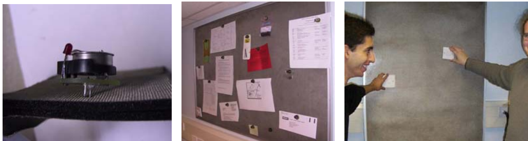
Figure 1: An implementation of the Pin&Play concept. From left to right: the networked surface and a pin-attached iButton computer; a smart noticeboard with more than twenty networked objects; and a demonstrator illustrating flexible placement of networked light switches on the wall.
