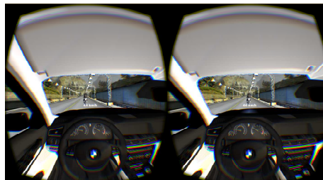
Figure 3: VR DS showing the sudden appearance of a motorcyclist in order to analyze the driver's reaction towards avoiding the head-on collision.
