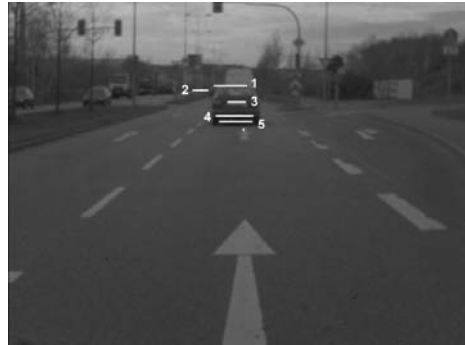
Figure 3: Example for the result of a Hough transform after LOC processing to extract line features (yellow lines thickened for visibility reasons)
